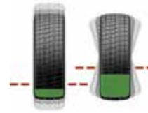
SmartWeight Balancing Technology® is a method of reducing forces on a wheel during balancing. SmartWeight® is not a procedure. Instead, it measures the forces of side-to-side movement and up-and-down shake and computes weight to reduce these forces. This reduces the amount of correction weight used, balancing time required, check spins needed and “weight chasing”.
